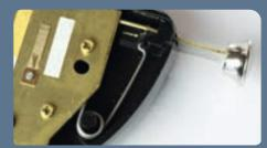
1. Simply put the spring over the plate to take away the tension.
